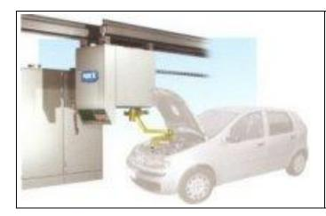
The unit is installed in car manufacturing factories where braking system are tested before new cars are sold.
