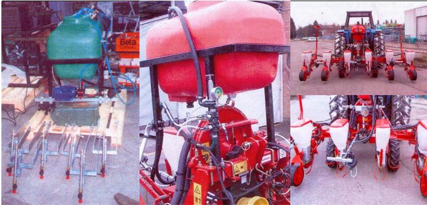
Equipment used for weedkilling. It is fit to sowing machines led by farm tractors and distributes liquids on the ground during the sowing process.
