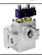
Press safety valves control the constancy of the flow of compressed air whenever compressed air becomes the power supply for the operation of pneumatic units. In order to carry out a safety function (complying with existing norms) the valves consist of a so called redundant system, a special surveillance circuit that stops the valve in case of air leakage in the net. The valve inhibits the operation of the electronic panel until the failure has been fixed and the pneumatic supply restored.
