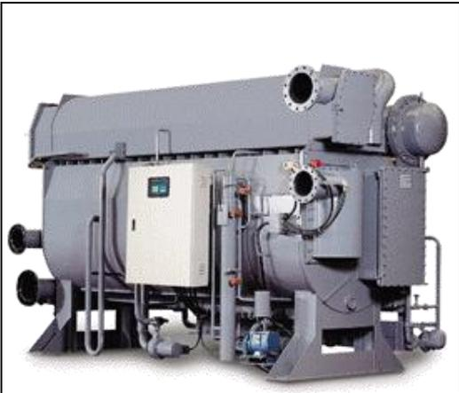
Chillers are cooling units for water and other process fluids. Thermal energy is turned into freezing energy by an absorption freezing cycle, in which the coolant changes its state in combination with the substance used as absorbent.
