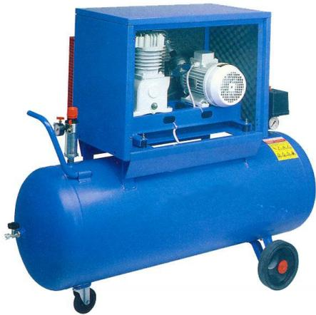
Machine used for the production of compressed air. It consists of a piston compressor with power supplied by an electric motor, a refrigerator and a tank. Its working principle is air compression: air is taken from the atmosphere, compressed by the compressor and collected into a tank. A filter is fitted at the intake to prevent foreign particles from going into the cylinder head. A cooling coil removes the condensate created by the heating of compressed air.
