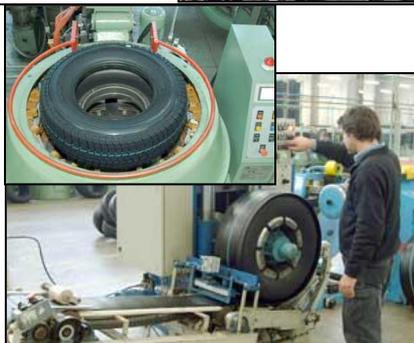
During the hot process the tread ring is smooth and is moulded in the curing press.
