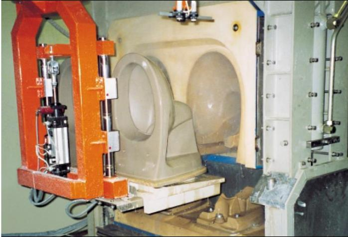
Industrial manufacturing of sanitary fittings such as rim bowls, wash basins, bidets or shower trays is carried out by high pressure casting systems. These systems are completely automatic and can carry out all production stages without manual interventions. The casting process consists of the following production stages:
