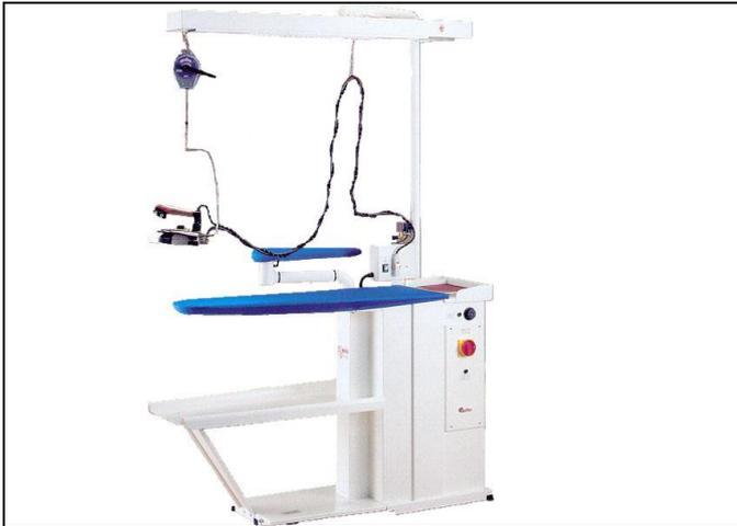
Integrated industrial ironing boards for the final finishing of clothing. The appliance is equipped with iron, vacuum blow table and sleeve form board. Ironing boards, utility presses and spotting tables make up an ironing group for various operators. Each machine can be self contained or connected to a steam, vacuum and compressed air set.
