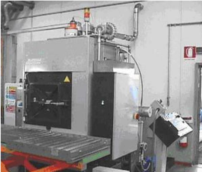
Metal cleaning machines are industrial cleaning machines with a closed-circuit drying system. They clean metallic parts of iron, aluminium, brass, bronze, stainless steel, etc. using solvents (ex. Perchloroethylene) and dry them with hot air. The cleaning operation can be carried out in three stages:
