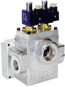
Press safety valves control the constancy of the flow of compressed air whenever compressed air becomes the power supply for the operation of pneumatic units. In order to carry out a safety function (complying with existing norms) the valves consist of a so called redundant system, a special surveillance circuit that stops the valve in case of air leakage in the net. The valve inhibits the operation of the electronic panel until the failure has been fixed and the pneumatic supply restored..
